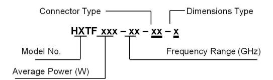
Please confirm with us the main parameters of terminations such as average power, frequency range, connector type and dimensions Type (if have any), or your special demand.
